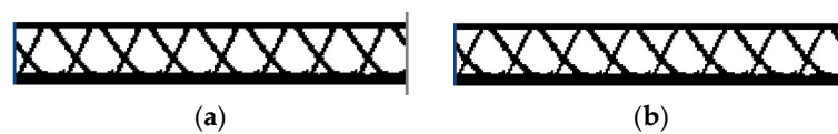
Figure 16. The cantilever T-beam results: (a) front view: only self-weight is considered; (b) front view: only distributed load P is considered.
