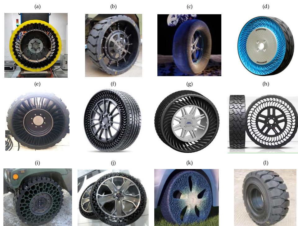
Figure 1. Representative examples of NPTs: (a) a high-load-capacity NPT [10]; (b) a mechanical elastic support type NPT [11]; (c) NASA’s Superelastic Tire made of a shape memory alloy [11]; (d) an Air Free Concept Tire [8]; (e) a Michelin Tweel [12]; (f) a Michelin UPTIS [7]; (g) a passenger car NPT designed by Jihua Laboratory; (h) i-Flex [9]; (i) honeycomb [13]; (j) an NPT with a negative Poisson’s ratio [11]; (k) a 3D-printed NPT [14]; (l) a solid-type NPT.
