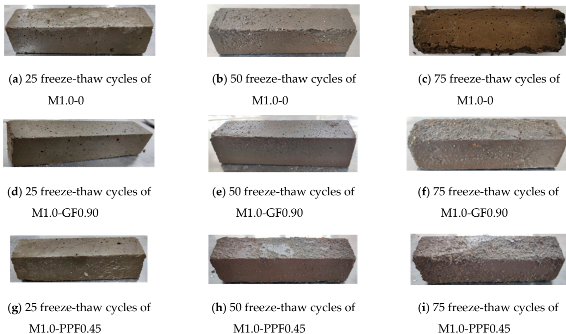
Figure 14. Surface morphology of freeze-thaw failure of mortar with alkali activator modulus of 1.0.
