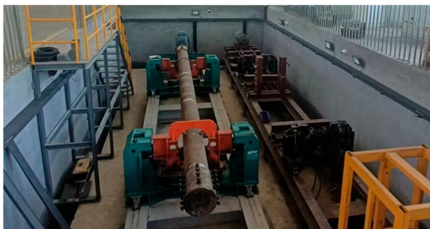
**Figure 2.** Resonance bending fatigue testing platform, Tianjin University (equipment no.: GWT0614; dimensions:  $15 \text{ m} \times 1.3 \text{ m} \times 2.0 \text{ m}$ ; range of the test pipeline diameter: 168.3–355.6 mm; range of the test pipeline length: 6–12 m; frequency: 0–25 Hz).
