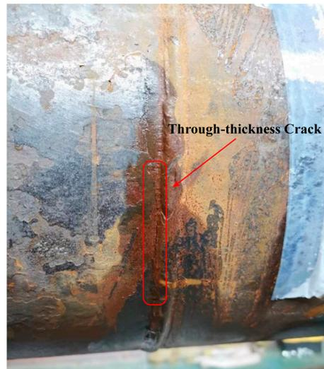
**Figure 3.** The occurrence of a through-thickness crack after internal water pressure leak.
