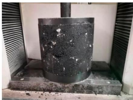
**Figure 1.** Unconfined compressive strength test.
