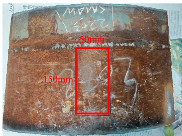
**Figure 5.** X80 pipeline steel specimen on post-service.
