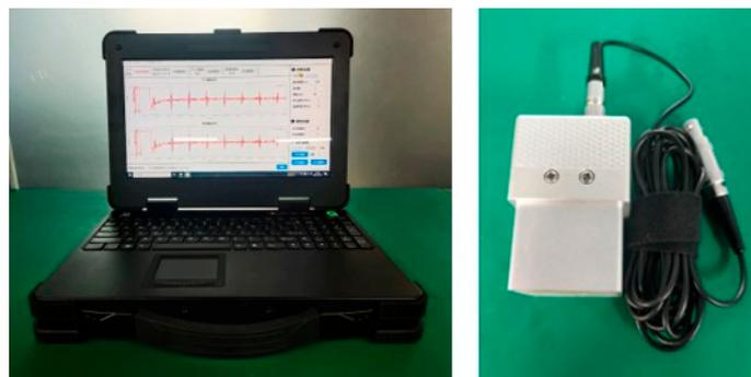
**Figure 2.** Residual stress measurement equipment and transducer of EMAT.
