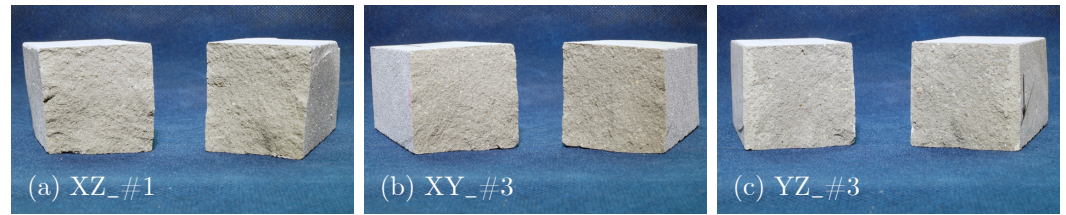
Figure 5. Fracture surfaces of 3PBT for Series I: specimens with layers oriented in (a) XZ-, (b) XY- and (c) YZ-direction.
