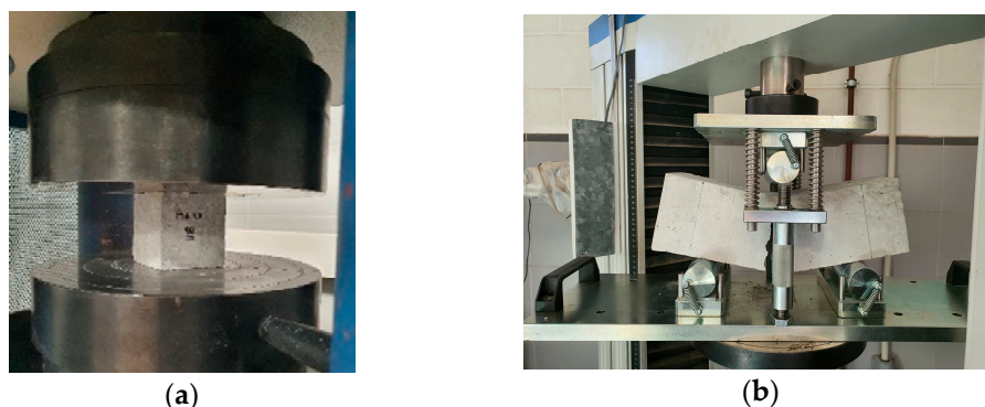
Figure 7. Strength tests of roller-compacted concrete: (a) compressive strength test; (b) flexural strength test.
