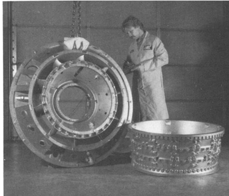
Figure 15. Large titanium engine component by Precision Castparts Corporation (reproduced with permission from Reference [320]; copyright © 2024 Published by Elsevier B.V.).
