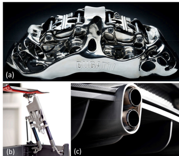
Figure 14. Bugatti titanium components: (a) eight-piston monobloc brake calliper, (b) active spoiler bracket, and (c) tailpipe trim covers (reproduced with permission from Reference [319]; copyright © 2024 The Authors. Published by Elsevier B.V.).
