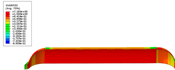
Figure 13. The whole fiber wrapping layer has almost completely failed.
