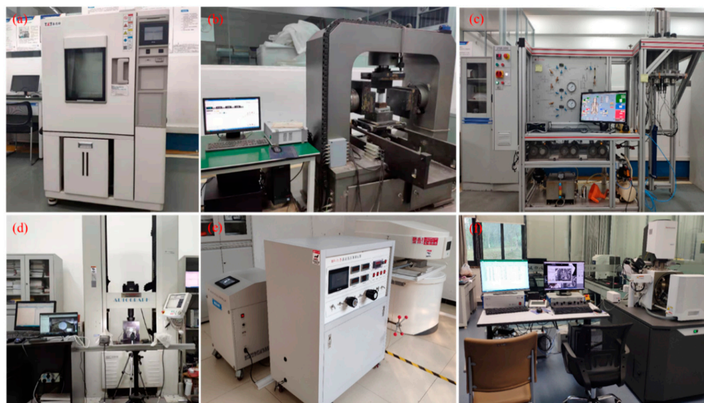
Figure 2. Main instruments: (a) high- and low-temperature alternating damp heat test chamber, (b) WDAJ-600 microcomputer-controlled electro-hydraulic servo rock shear rheological test machine, (c) ROCK600-50HTPLUS multifunctional rock full stress triaxial test system, (d) AG-250kN IS precision electronic universal material test machine (e) non-destructive NMR system for rock core imaging and analysis, and (f) field emission transmission electron microscope.
