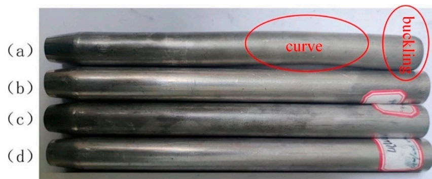
Figure 3. Necking parts of the 5A02 aluminum alloy tube under different current intensities: (a) I = 100 A; (b) I = 200 A; (c) I = 300 A; (d) I = 400 A.
