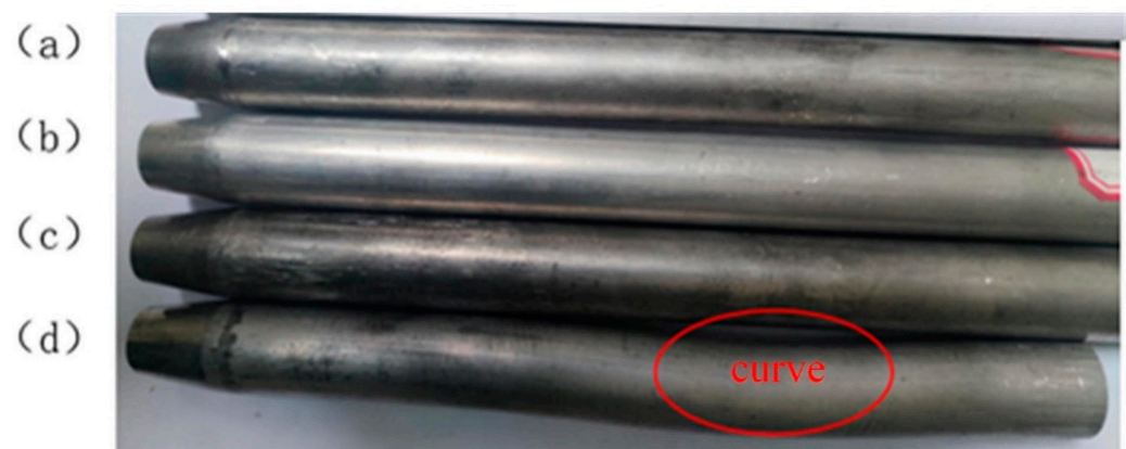
Figure 10. Necking parts of 5A02 aluminum alloy tube at different feed speeds: (a) v = 2 mm/min; (b) v = 5 mm/min; (c) v = 10 mm/min; (d) v = 20 mm/min.
