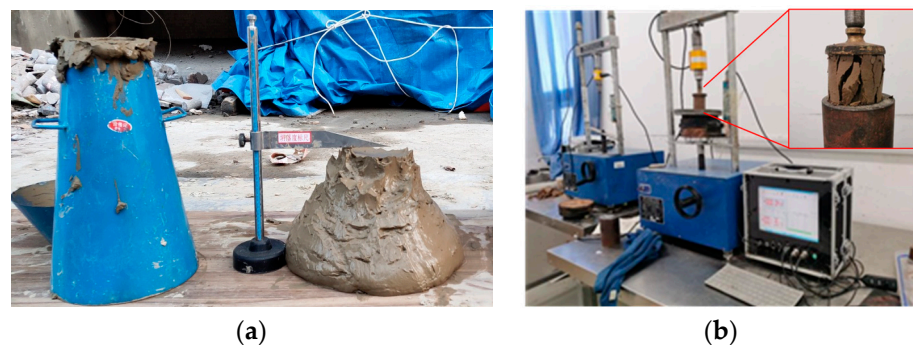
Figure 3. (a) Slump cone and (b) CBR-2 testing equipment with damaged specimen.
