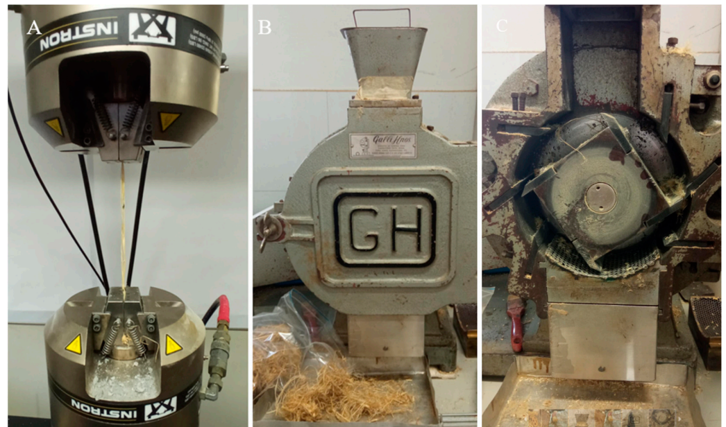
Figure 14. (A): Hemp fiber tensile strength measurement, (B,C): blade mill used for cutting fibers.
