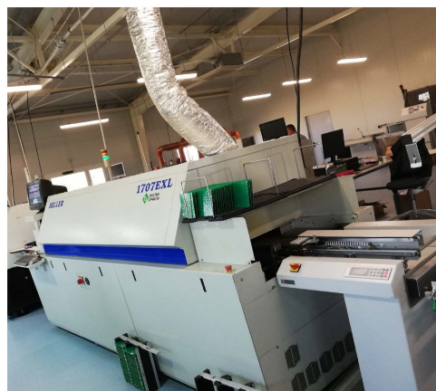
Figure 1. Industrial oven from MIBATRON S.R.L utilized for reflowing of Sn-Cu-Ni ternary alloy.
