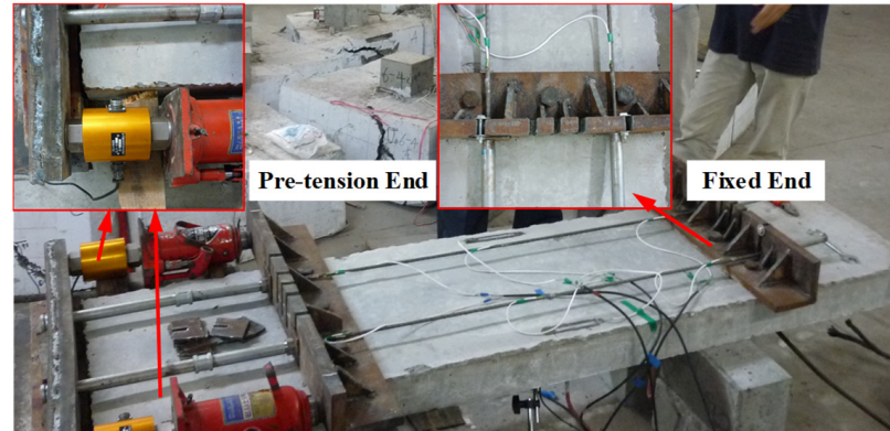
Figure 2. Anchoring and prestress tension of GFRP bars.
