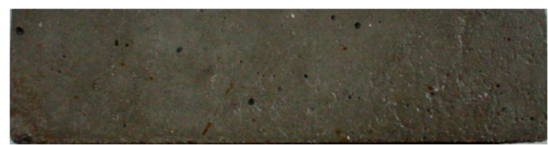
(b) SFRHSEC after freeze–thaw cycles (30% RH)
