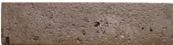
(c) SFRHSEC after freeze–thaw cycles (50% RH)
