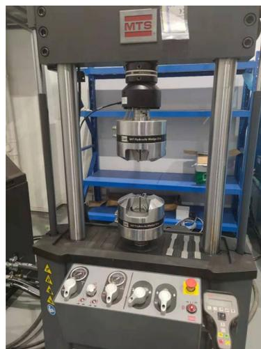
**Figure 2.** MTS fatigue testing machine.
