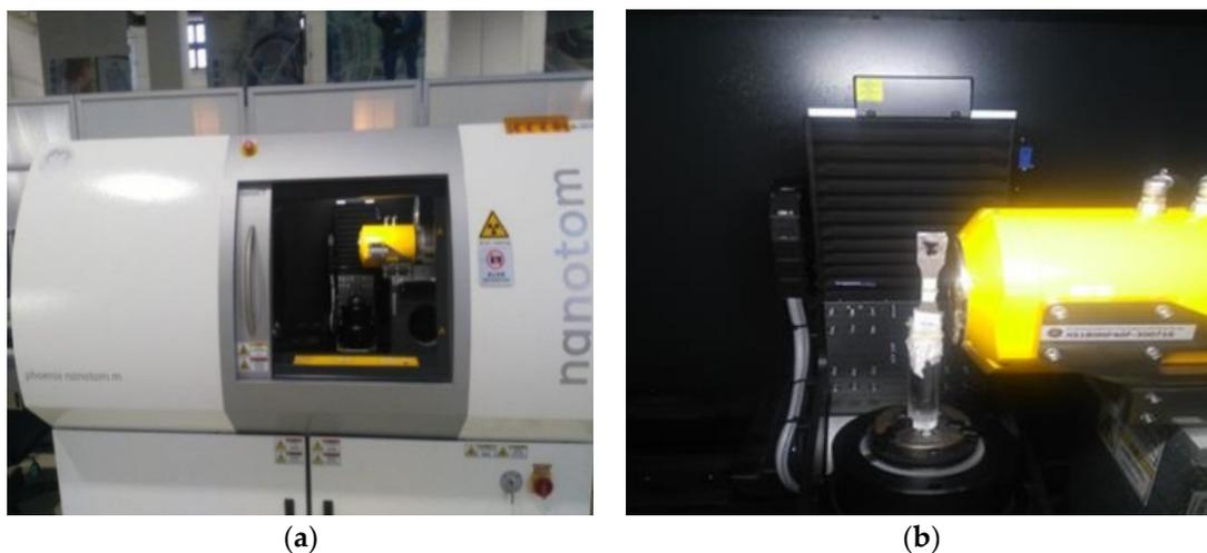
**Figure 4.** CT scanning device. (a) CT-Phoenix nanotom. (b) X-ray emitter.
