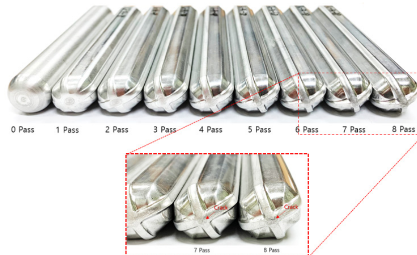
Figure 16. Appearance of workpieces depending on the number of forging passes.
