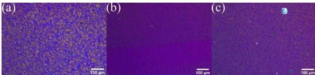
**Figure 16.** Metallographic structure of RZ in (a) 0.5% (b) 1% (c) 2% GNS-reinforced AMC.
