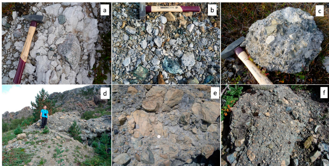
Figure 2. Field photos of M-(A)-S-H cemented till and moraine. (a–c) Feragen and (d–f) Leka.
