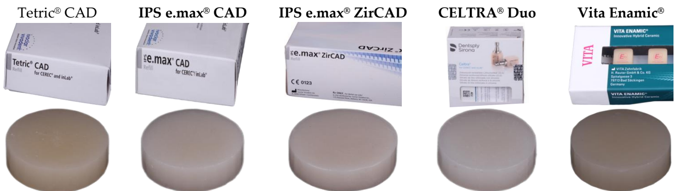
Figure 1. Test materials with their corresponding specimens (10 mm diameter and 3 mm thickness).
