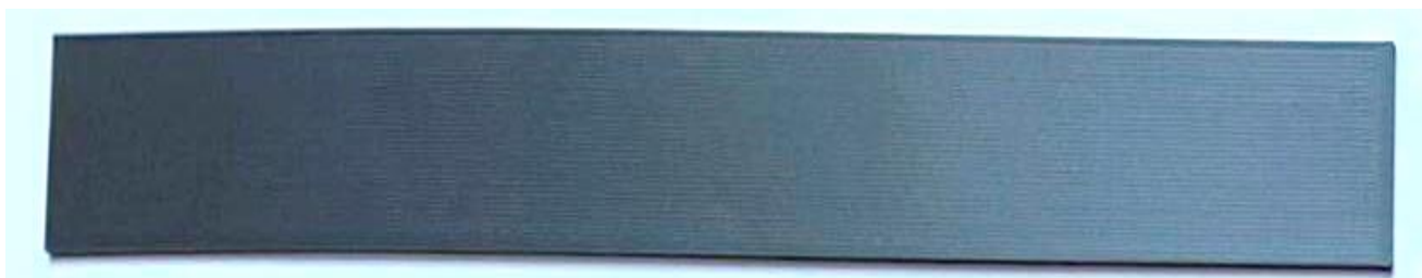
Figure 4. Example of PC blend carbon fiber lamella.
