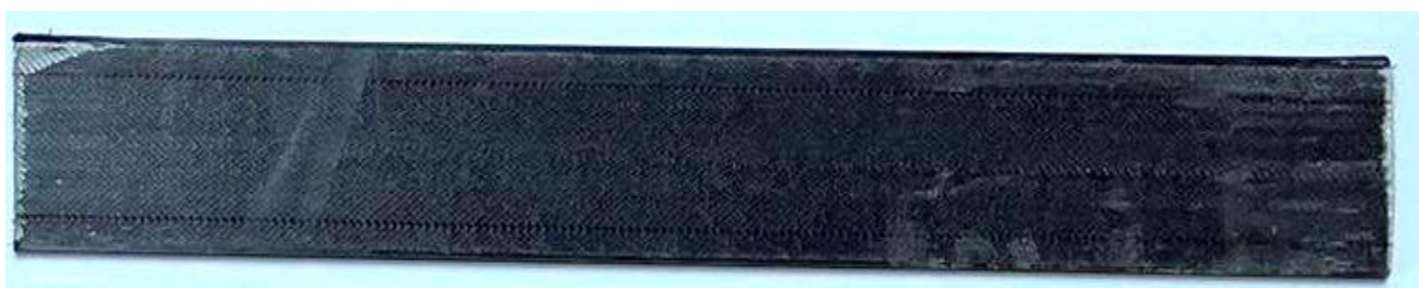
Figure 2. Example of a CFRP lamella.
