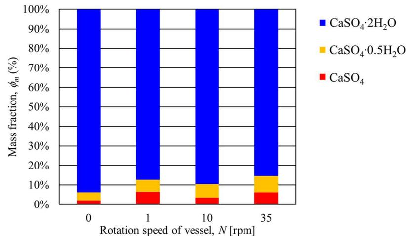
**Figure 6.** Relationship between the transferring mass fraction of gypsum and the rotation speed of the rotary vessel at a heating end temperature of  $100^\circ\text{C}$ .
