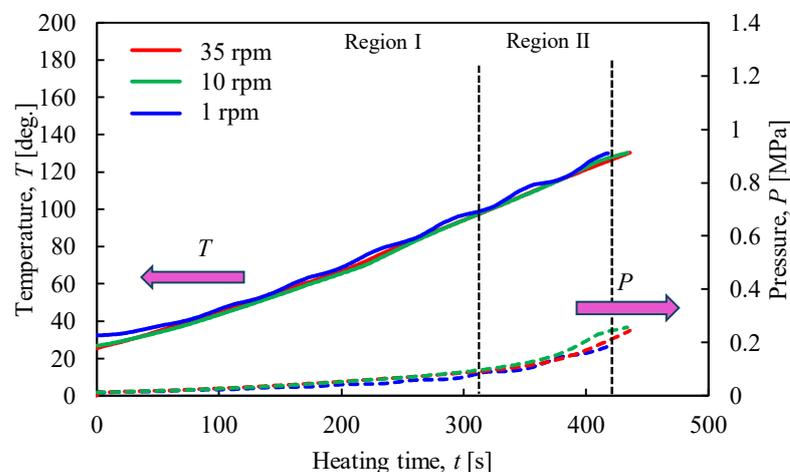
**Figure 7.** Time histories of temperature and pressure inside the rotary vessel at a heating end temperature of  $130^\circ\text{C}$  when the rotation speed was changed.
