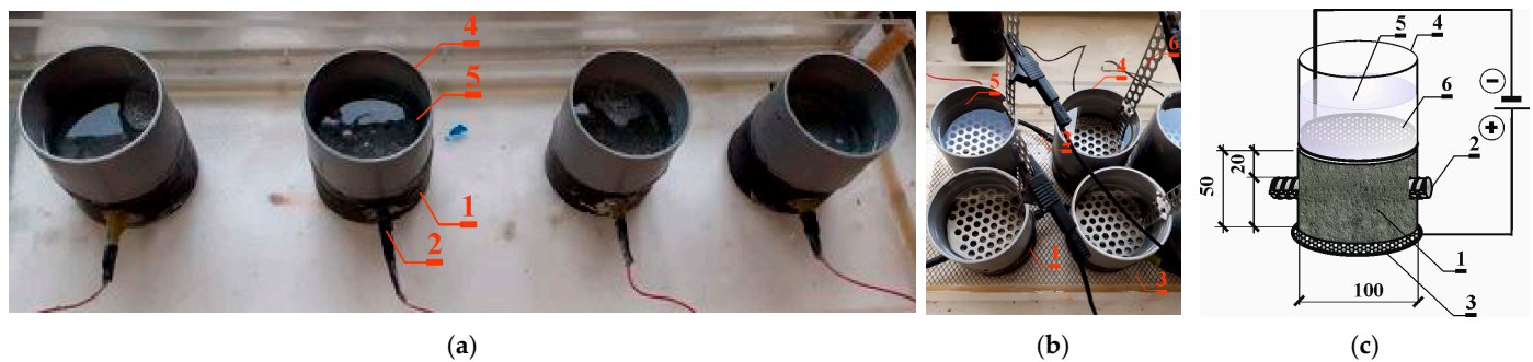
Figure 1. (a) Samples prepared for testing from C1 concrete. The experimental setup for accelerating the migration of chloride ions to concrete through the application of an electric field. (b) Research view. (c) Schematic image of the study: 1—concrete test specimen, 2—ribbed rebar \varnothing 12 mm made of steel B500S, 3—titanic anode coated with platinum, 4—small plastic tanks with 5—3% NaCl, 6—stainless steel cathode.
