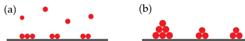
Figure 3. Volmer–Weber model: (a) creation of clusters; (b) clusters of deposited material.
