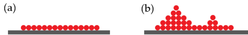
Figure 4. Frank–van der Merwe model: (a) creation of monolayer; (b) 3D islands of deposited material.
