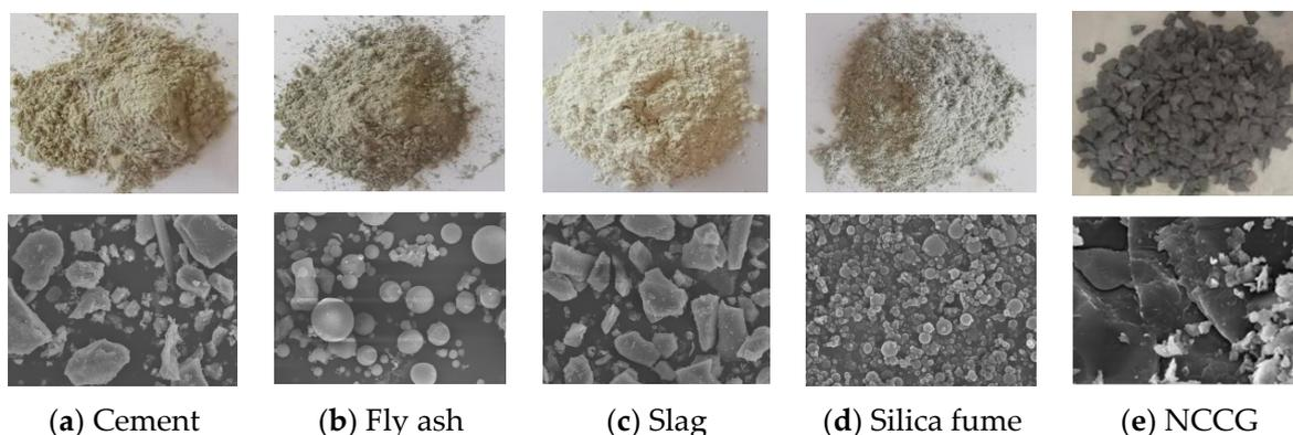
**Figure 1.** Raw materials and their SEM photos (Magnification factor 2000×).
