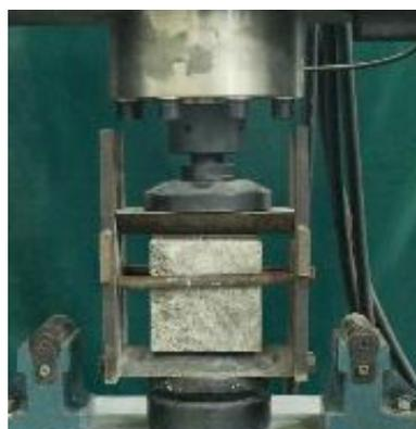
**Figure 3.** Splitting tensile strength test device.
