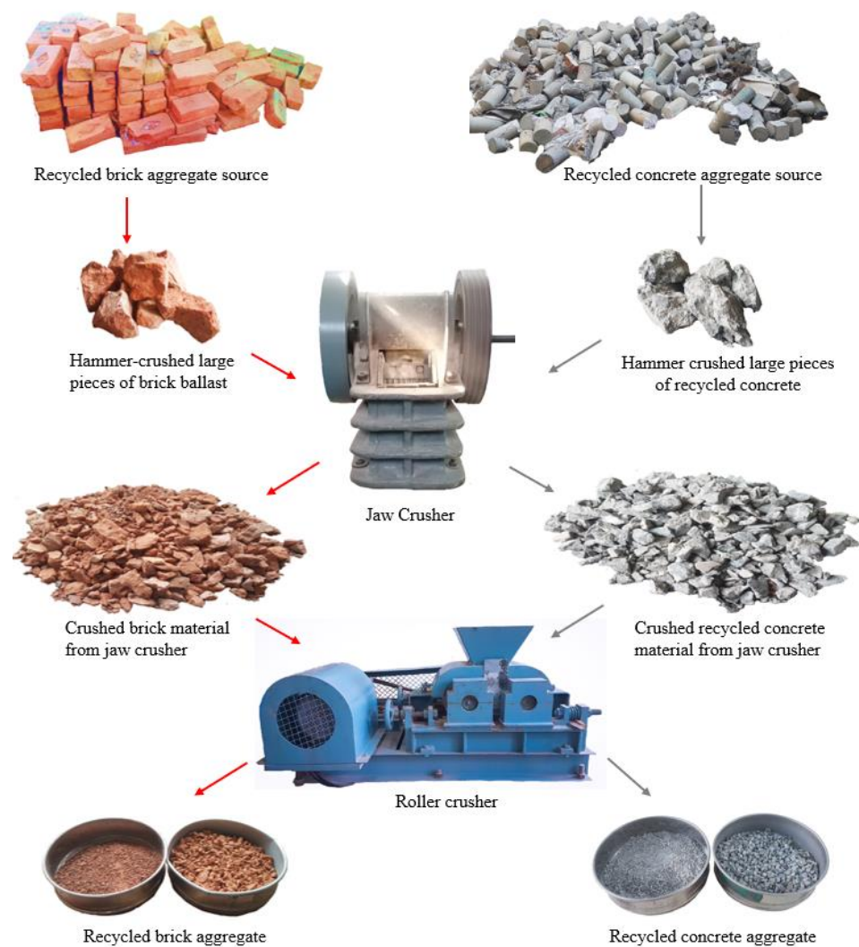
Figure 4. Production process of recycled aggregates.
