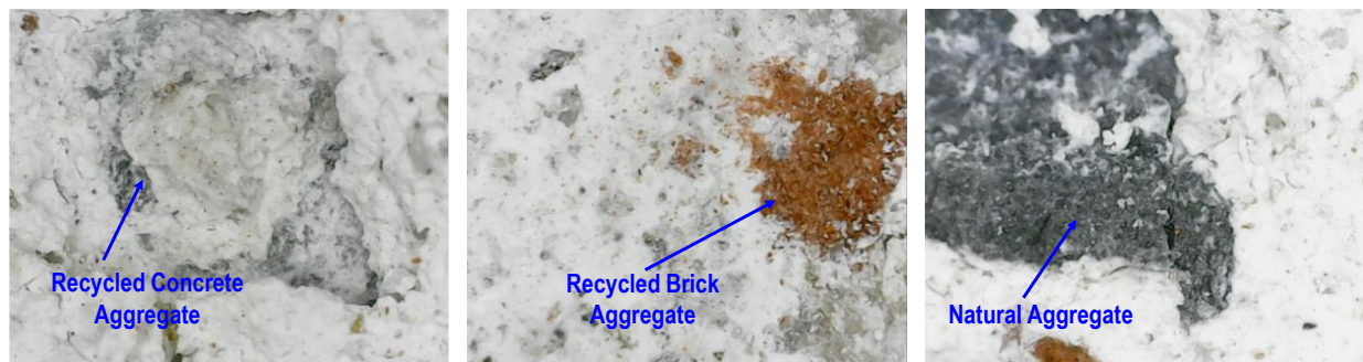
Figure 19. Gypsum formation on the surface of concrete specimens after four cycles.
