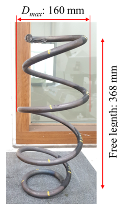
Figure 1. Geometry and dimensions of spring specimens.
