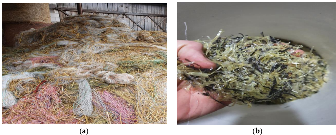
Figure 1. Waste netting for bale wrapping: (a) heaps of used netting at the farm and (b) netting in the form of fibres as dispersed reinforcement in the designed composites.
