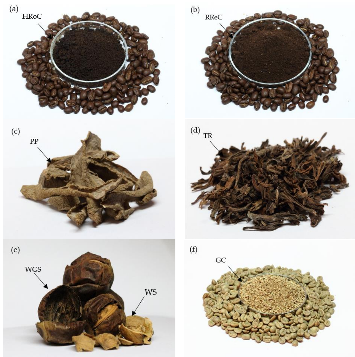
Figure 2. The collected and pre-prepared organic waste, used for the preparation of bioadsorbents: (a) heavily roasted coffee residue, (b) regular roasted coffee residue (c) potato peelings, (d) tea residue, (e) walnut green shells and walnut shells, (f) green coffee residue.
