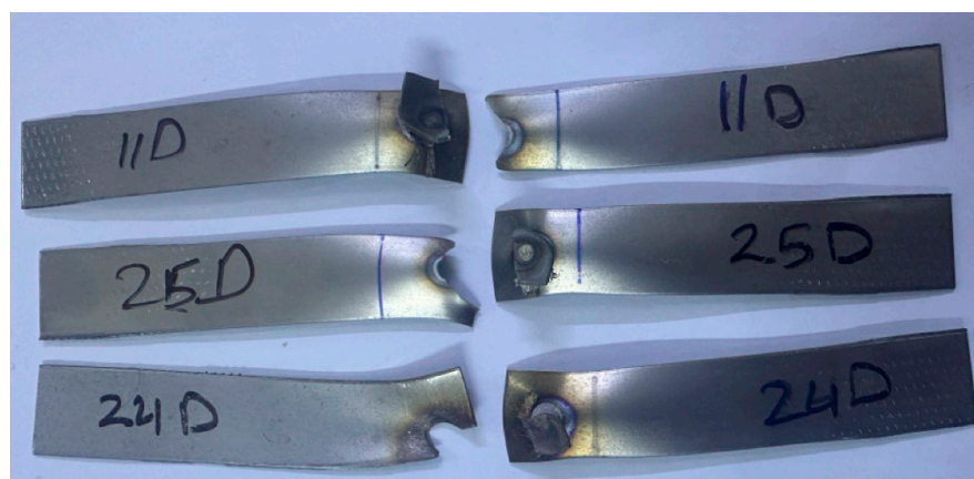
Figure 24. Crack transferring through the width in case D.
