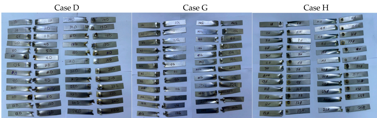
Figure 4. Fractured resistance spot-welded specimens after the tensile test.
