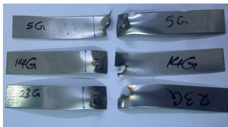
Figure 26. Crack transferring through the width in case G.
