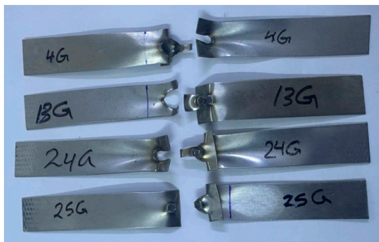
Figure 25. Complete withdrawal of the nugget in case G.
