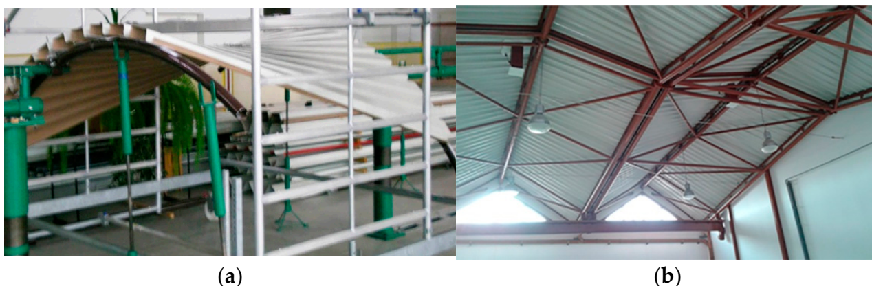
Figure 1. Directrices defining the transformations of roof coverings made of thin-walled trapezoidal sheets nominally flat and corrugated in one direction: (a) experimental tests; (b) the roof of the laboratory hall used in the previous tests (our own photos).
