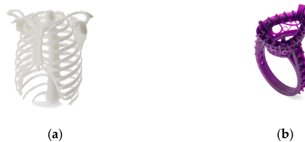
Figure 7. Examples of SLA products, (a) model of ribs and spine (b) ring model.
