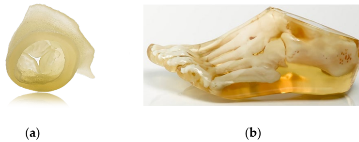
Figure 9. Examples of Poly Jet products (a) valve model (b) foot model.
