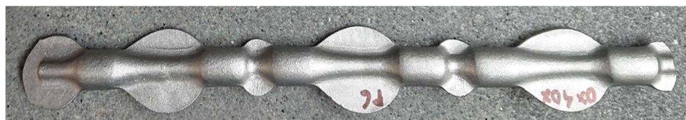
Figure 21. A semi-product made as a result of reforming of the charge material in the form of a bar on the pre-roughing pass 0X.
