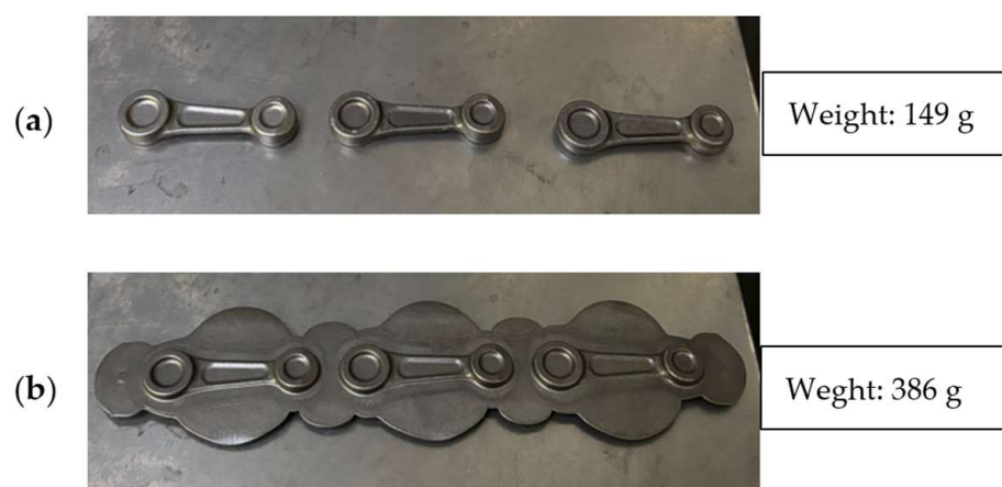
Figure 6. Views of a connecting rod forging: (a) a forging after trimming the flash, and (b) a forging with a flash.
