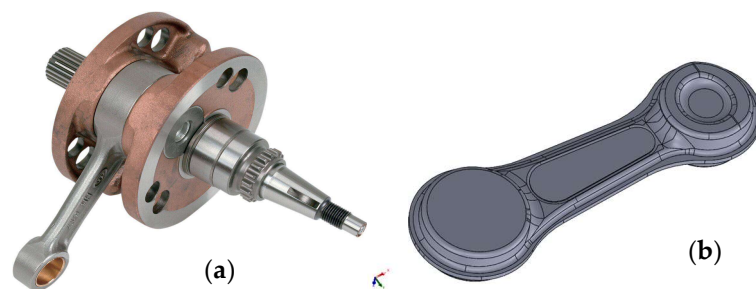
Figure 1. The view of (a) the solid of the complete crankshaft, and (b) a 3D drawing of the connecting rod.
