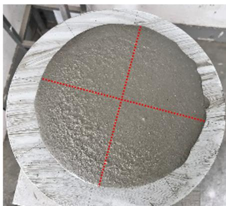
**Figure 1.** Mortar fluidity test.
