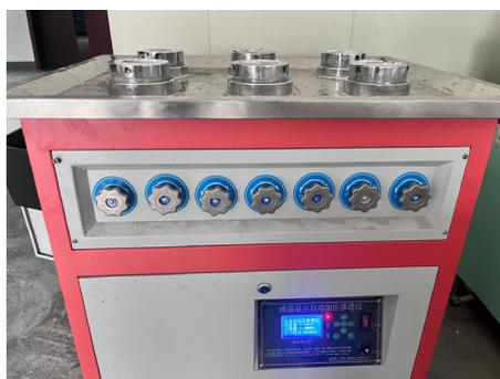
**Figure 5.** Automatic pressure permeability apparatus. The non-English terms pertained to the operational precautions for the testing apparatus.
