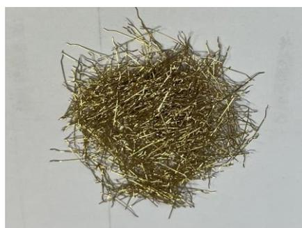
**Figure 4.** Photograph of steel fiber.
