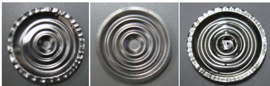
Figure 28. Appearance of semi die formed samples using 12 J (L), 15 J (M) and 18 J (R) [70].
