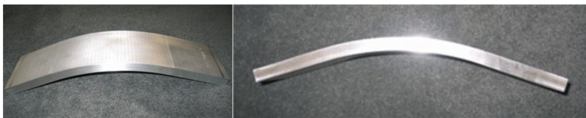
Figure 25. A 0.4 inch (10 mm) thick piece of Aluminum 7050 formed by laser peening [47].
