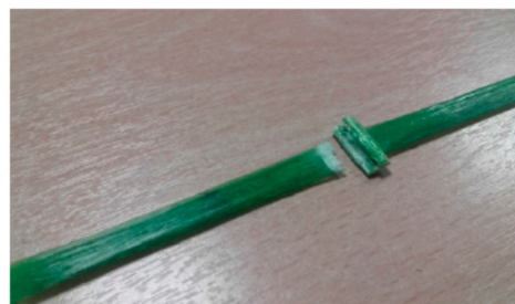
Figure 10. Partial fiber-failure at the GFRP grids joint.
