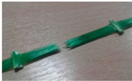
Figure 9. Catastrophic collapse of the GFRP sample.
