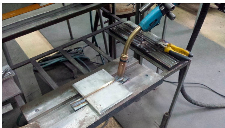
Figure 2. Components and welding torch.
