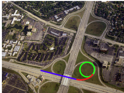
Figure 3. Rotation curve. The transition between the straight part (blue) and circular part (green) is a spiral curve (red). Picture is taken from https://cifrasyteclas.com/clotoide-la-curva-que-vela-por-tu-seguridad-en-carreteras-y-ferrocarriles/ .
