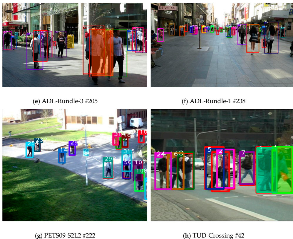
Figure 3. Exemplary qualitative tracking results for the MOT15 benchmark dataset. (a–d) are from a set of training images and (–h) are from a set of testing images. Following # is the individual frame number in each image sequence. Different trajectories are illustrated in different colors, with different identities marked in white. The red boxes without identities are detections, some of which have not been associated with trajectory. The filled boxes are low-confidence trajectories, while the unfilled rectangles are high-confidence trajectories.
