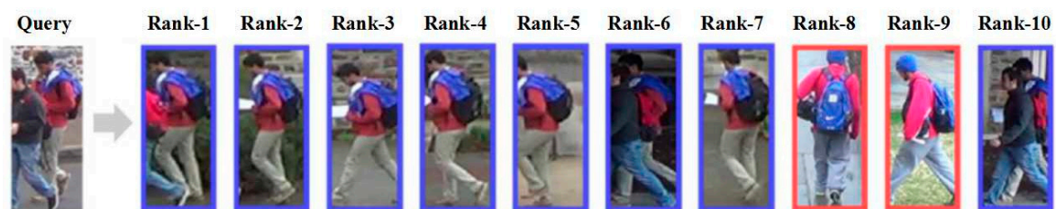
Figure 7. One example query image in DukeMTMC-reID dataset and ranking list results from Rank-1 to Rank-10 using MFF model. The blue boundary means true positive and red means false positive.
