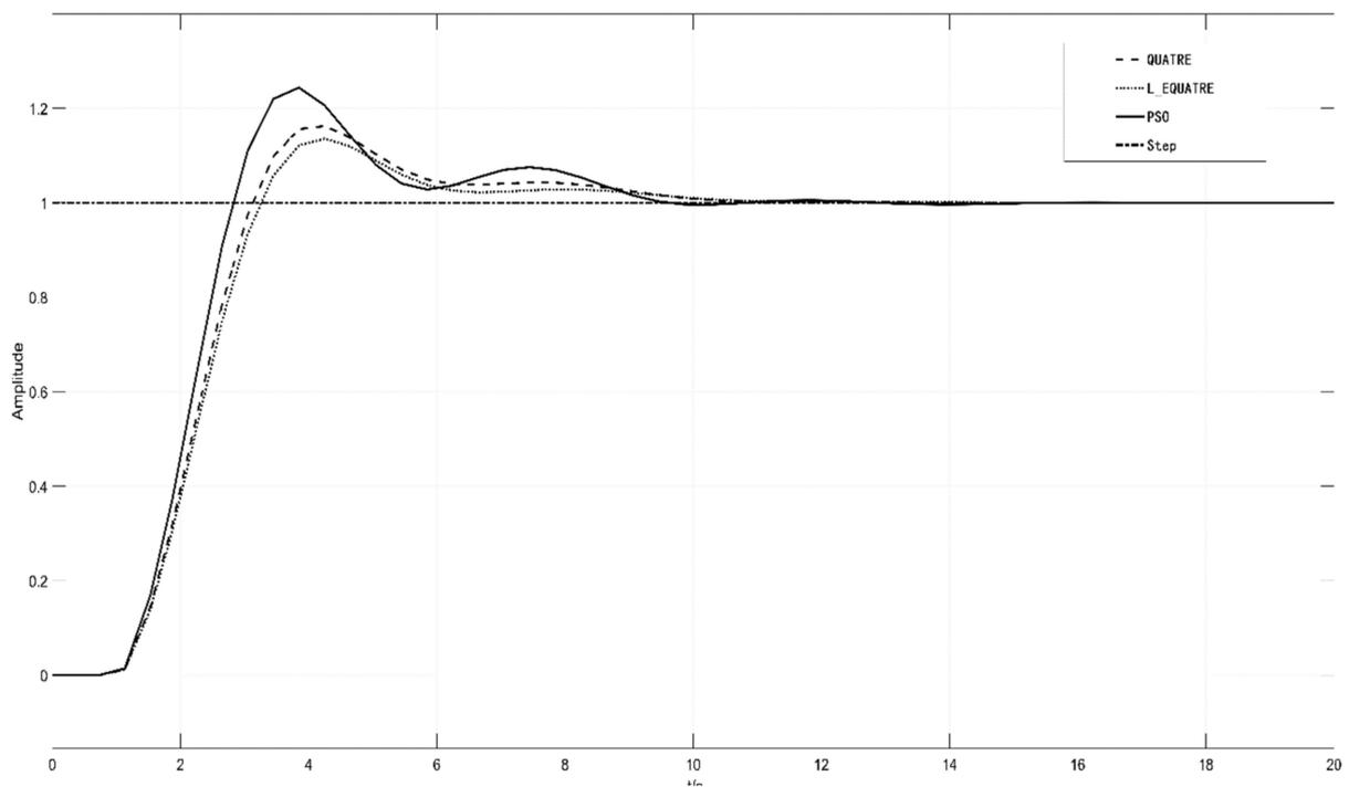
Figure 7. The unit response curve of the second-order controlled object.
