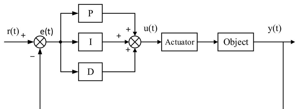
Figure 1. PID control schematic diagram.
