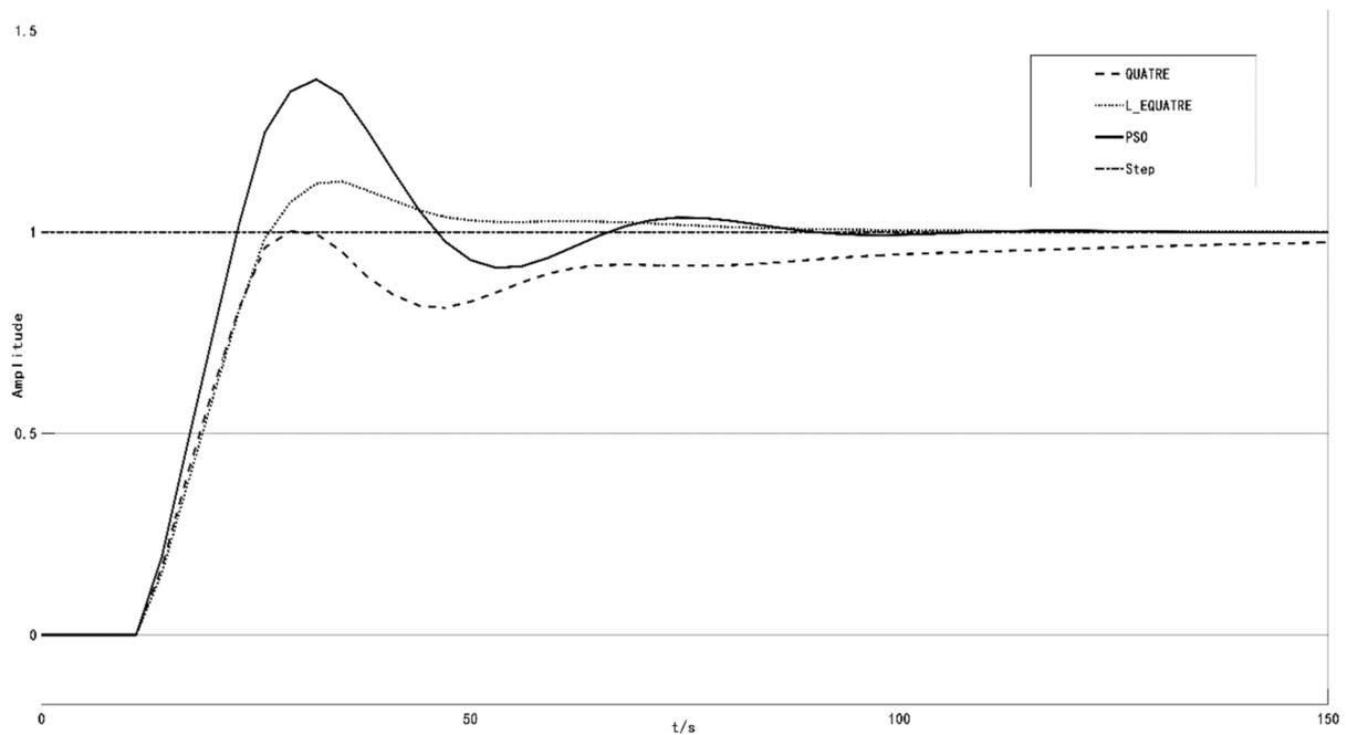
Figure 6. The unit response curve of the first-order controlled object.
