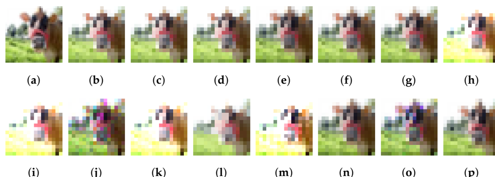
Figure 9. The CIFAR100 horse original image (a) and the respective results of the first pass of pooling for the methods Max (b), adaptive Max (c), fractional (d), Average (e), mixed (f), gated (g), tree (h), l2 (i), stochastic (j), fuzzy (k), overlapping Max (l), spectral (m), wavelet (n), LIP (o) and SoftPool (p).
