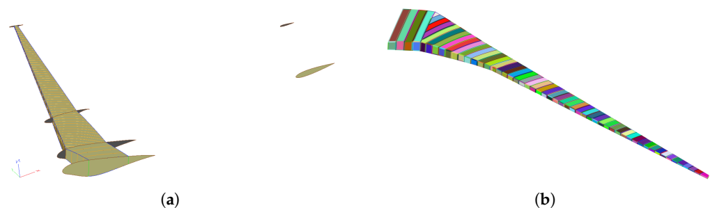
Figure 2. ESP parameterization of the uCRM. (a) ESP geometry used for LF analyses showing designable airfoil shapes at the wing Yehudi and tip. (b) Faces of IML geometry components with varying thickness (color variations only used to denote different components).
