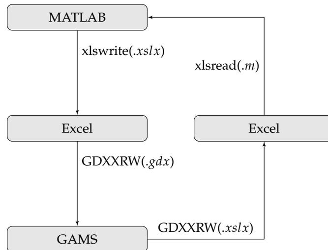
**Figure 1.** Diagram of the information exchange in the MATLAB–GAMS interface.
