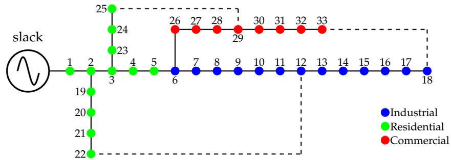
Figure 3. Electrical diagram of IEEE 33-node meshed test system.
