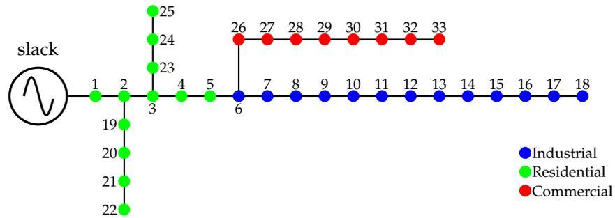
Figure 2. Electrical diagram of the IEEE 33-node radial test system.
