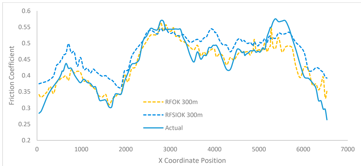
Figure 9. ML hybrid model performance at a separation distance of 300 m.
