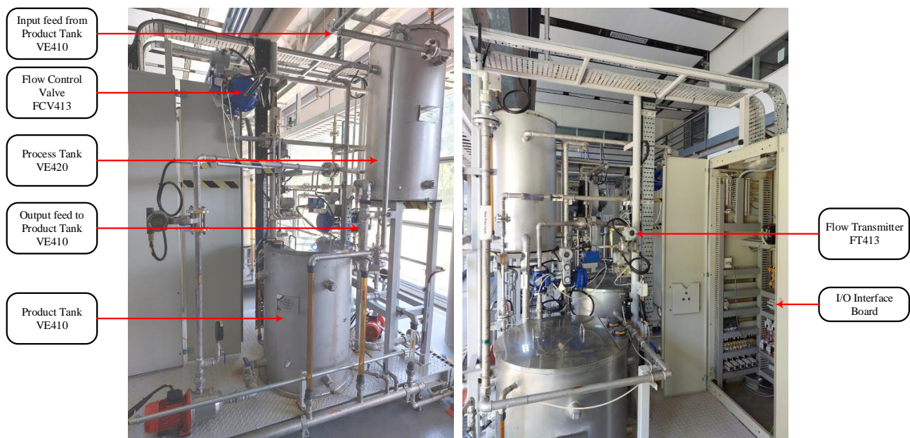
Figure 26. Schematic of real-time flow process plant.
