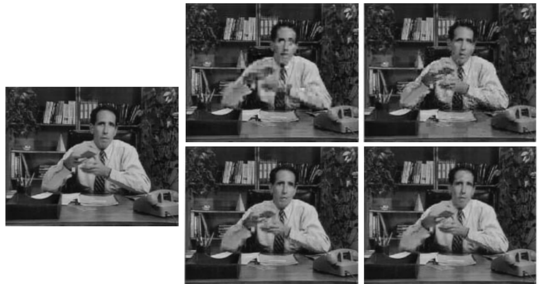
Figure 1. Examples of video compression using 3D DCT, comparing the original video frame and various compression techniques, with variable-temporal-length 3D DCT implementations in the bottom row, clearly showing its superiority.
